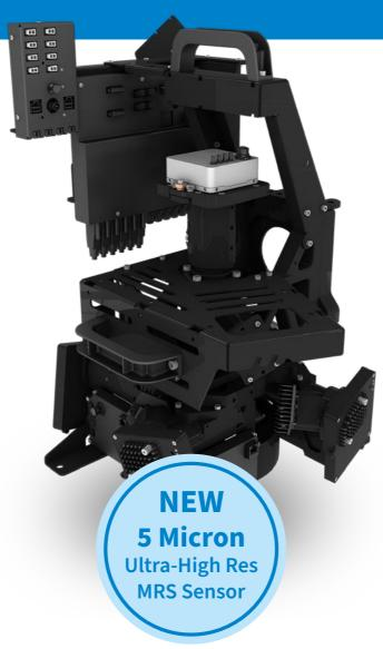
The SQ3000+ is powered by Nordsons' proprietary 3D sensing technology with sophisticated fusing algorithms that enables metrology grade accuracy at production speed. The result is ultra-high quality 3D images, high-speed inspection and metrology, and improved yields and processes.
