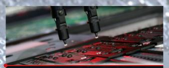
Multi flexible feeder, multi lane cassette or highly accurate single lane feeder. Tape, Stick, Strip, Tray slider. Largest component spectrum; 01005 up to 80 x 80 mm, component height up to 25 mm.
