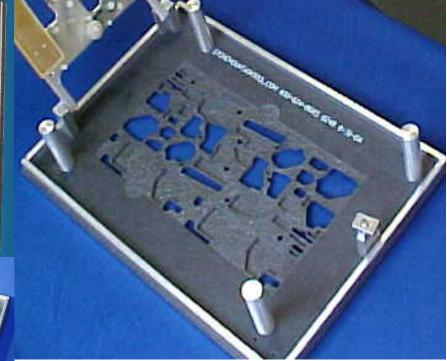
Selective soldering pallets allow the soldering of plated through hole (PTH) components to dual sided mixed technology assemblies while protecting solder side surface mount devices (SMD). These pallets have
