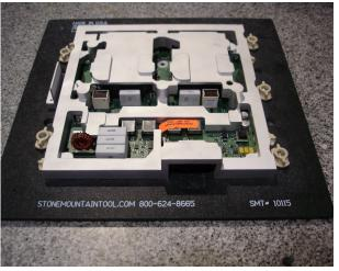
Pallets used in conformal coating provide clearance for over hanging components, masking of board or component areas, and are cleared to direct overspray downward to the machine filter system and <u>not</u> on your expensive conveyor system. Pallet materials are resistant to coating solvents for easy cleaning in a dip pan. Conformal coating pallets are a cost reduction method for machine down time due to cleaning and elimination or reduction in manual masking operations.
