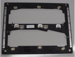
Open aperture pallets are the earliest form of fixtures for the wave solder process. They provide parallel and even edges, flatness stability to the process, clearance for overhanging components, edge masking, a common conveyor width across your production mix, and other unique features required of your specific application.
