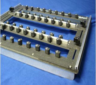
Super heavy duty, Stainless Steel wash trays are made from 16 ga., perforated sheet. They are welded, corner braced, and hemmed for operator safety. A unique fine mesh Stainless Steel drape lid is utilized to minimize PCA movement during washing. The lid is retractable and is provided with a convenient locking lift handle mounted to a lid stiffener. Trays can be custom fabricated to any size and depth.
